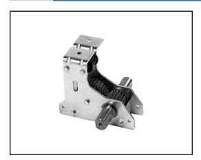
The THG40 rack box forms part of a screen system and is mounted under the truss. The rack box is driven by a GW motor gearbox and drives the pull-push tube by means of a gear rack.
