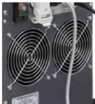
Detail of the control panel, with cooling fans and connection to the remote control of Fog Innox Multi Ambiente module
